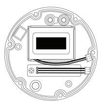
8. Remove the cushion and attach it to the new battery and reconnect the connector. Make sure the o-ring is positioned correctly before reinstalling the screws. Follow pattern below when tightening the screws.
