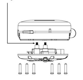
6. Should the springs pop out set them aside while replacing the battery.
