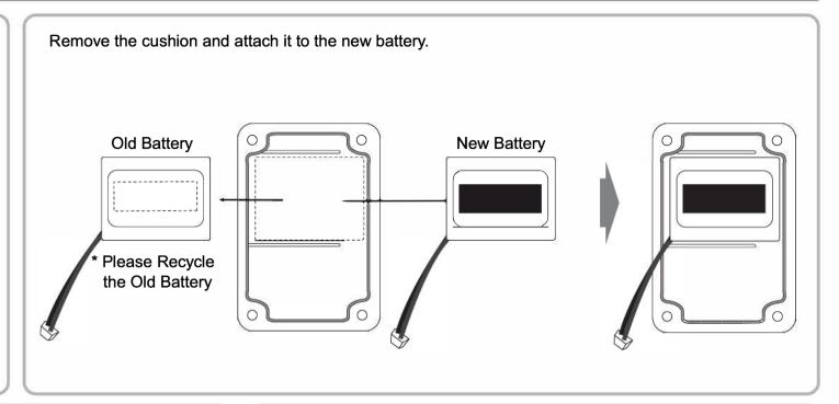
Reinstall new battery and reconnect the connector. Be careful to keep the wire away from transformer.
