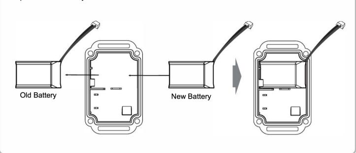
Reinstall the new battery and reconnect the connector, taking care to keep the wire away from the transformer.
