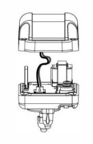
Be careful not to pinch the wire, as shown in the figure below, to avoid causing a broken wire.
