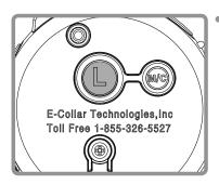
To turn the Transmitter On or Off : Press the "L" button for more than 1 second.
